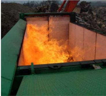
**General:** A self-contained, completely assembled above ground Air Curtain Burner (air curtain incinerator or FireBox) with a refractory lined burn-container for portable and permanent (stationary) applications. Designed for the high temperature burning of forest slash, land clearing debris, green waste, storm debris, and other waste streams in compliance with the requirements of US EPA 40CFR60.
